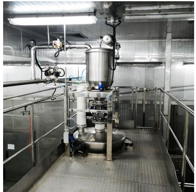
TRC 70.18.500.700 Compact BF 3 in 1 Coffee Receiver Filling Machine Application
